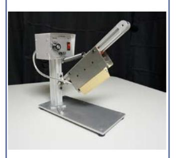
Model shown: RX-80-BAL-RK 5" Heavy-duty Brass Knife, 120V (see custom configurations on back)
